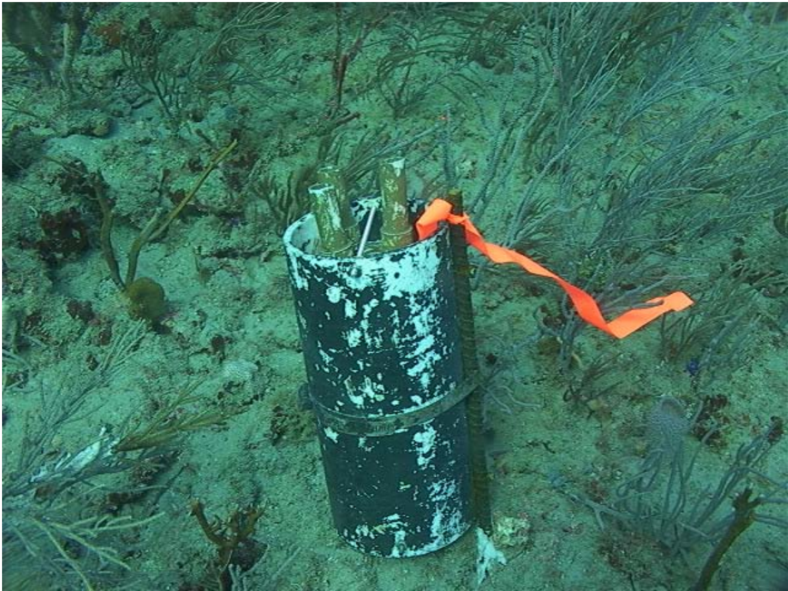
Figure 8.2. Sediment trap permanently installed at each end of a monitoring transect.
